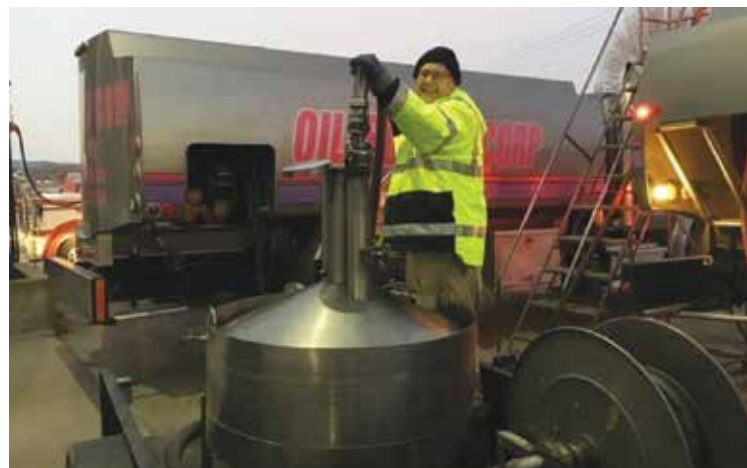
Inspector Dwight Brunette testing a Vehicle Tank Meter in the early morning hours.
