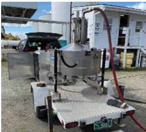
Weights & Measures 100-Gallon Testing Unit (Prover)
