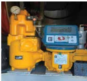
Vehicle Tank Meter used for commercial fuel deliveries.
